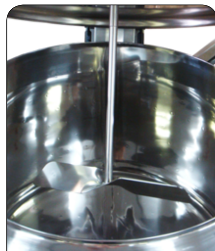
Polished interior of the kettle (mirror)
