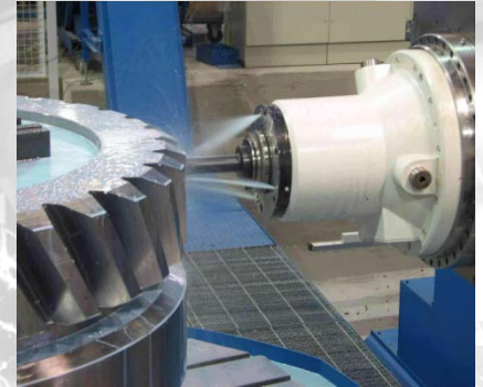
Gear cutting by milling technology (recommended for gear diameter 4 – 10 m)
