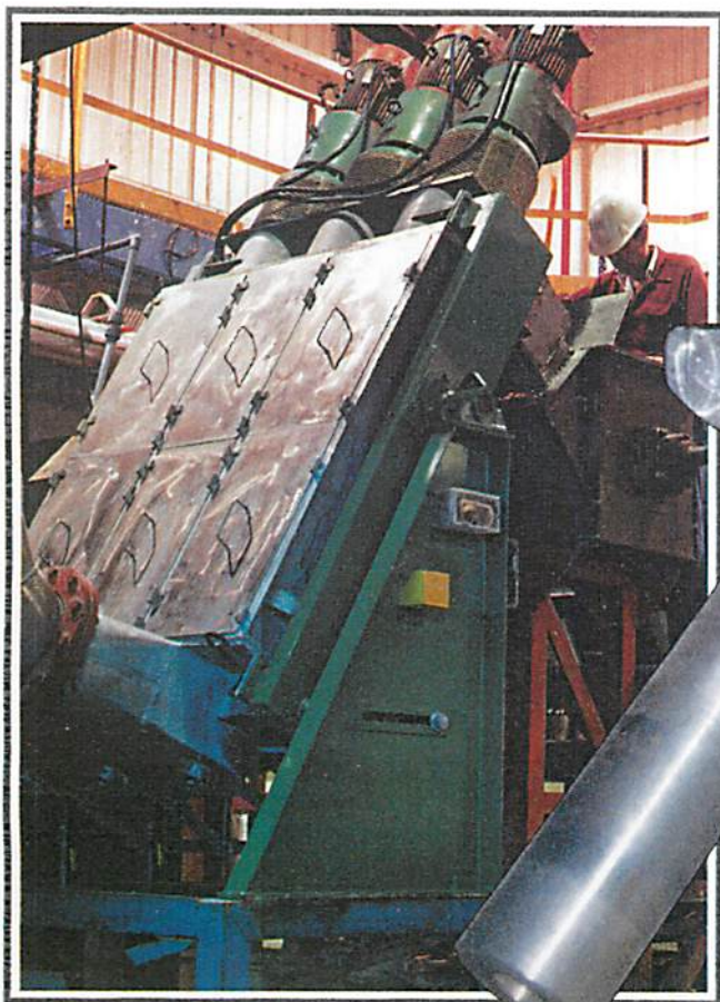
Typical deinking tissue mill employing Hymac extractors for washing.
