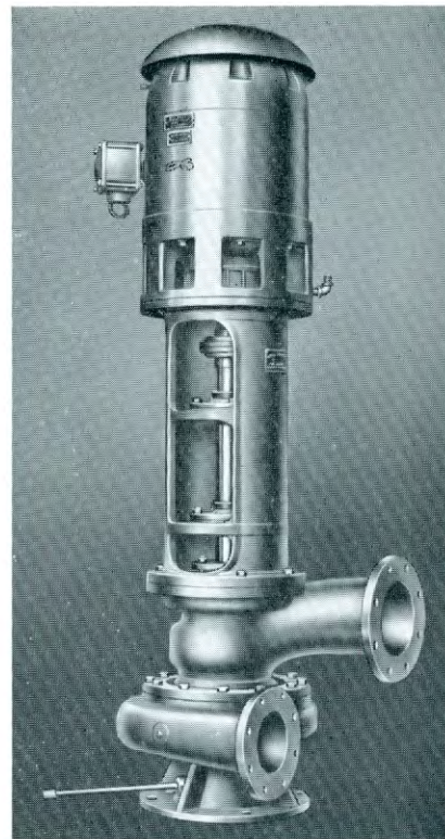
Fig. 309. Vertical top suction non-submerged "HBD" pump with outside liquid sealing well for handling hot volatile liquids. See bulletin D-85 for other "HBD" vertical pumps.
