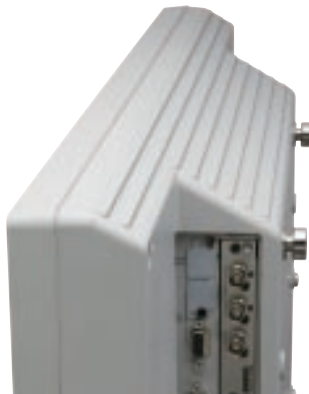
Ventilation holes (Side view)
