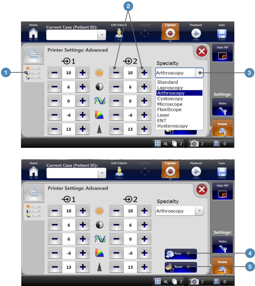
1. Selecting the **ADVANCED SETTINGS** tab navigates to the “Printer Settings: Advanced” screen.
