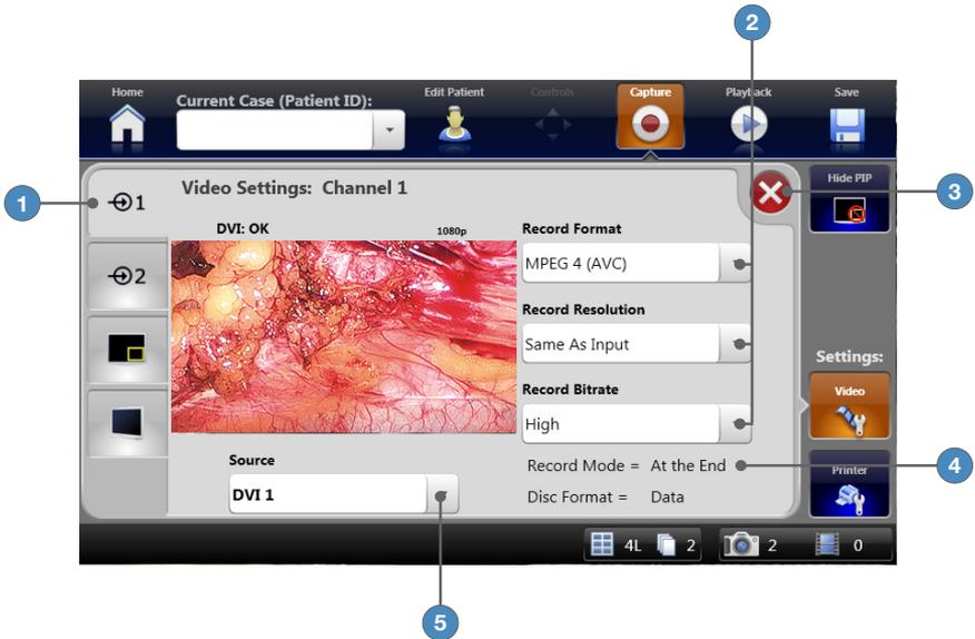
1. Pressing the **CHANNEL 1** tab displays the "Video Settings: Channel 1" screen.
