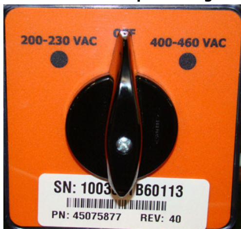
Figure 1-3: Main AC input voltage switch
