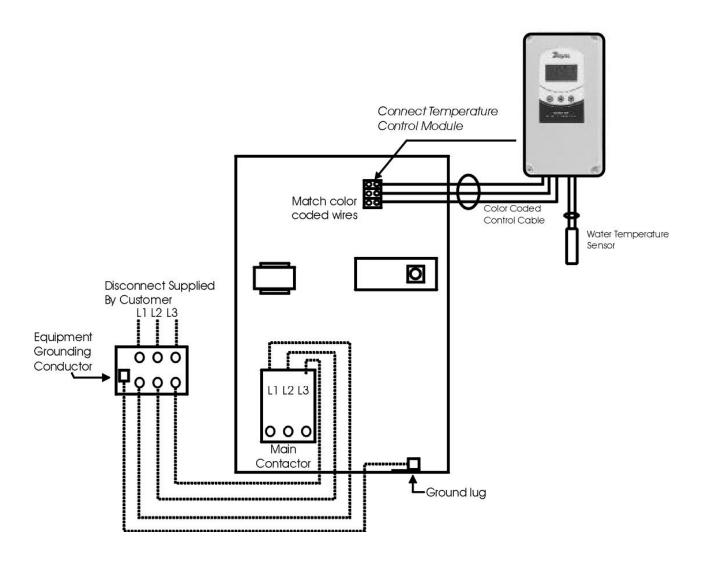
**Electrical Diagram Without Hot Gas By-Pass**
