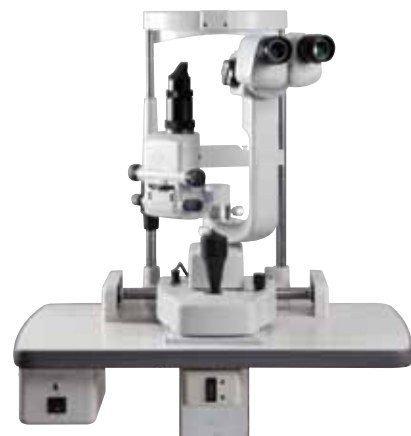
SL-D4 Five Magnification Digital Slit Lamp The SL-D4 incorporates a parallel drum magnification changer that allows for quick selection among five convenient magnifications of 6X, 10X, 16X, 25X and 40X. The 40X magnification is especially useful for Corneal Endothelium observation. Encompassing a variety of ophthalmic applications, the demanding eye care specialist can produce excellent images of both anterior and posterior structures of the eye.
