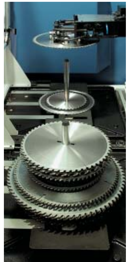
With two loading carriages for approx. 50 saw blades with three loading carriages for approx. 100 saw blades
