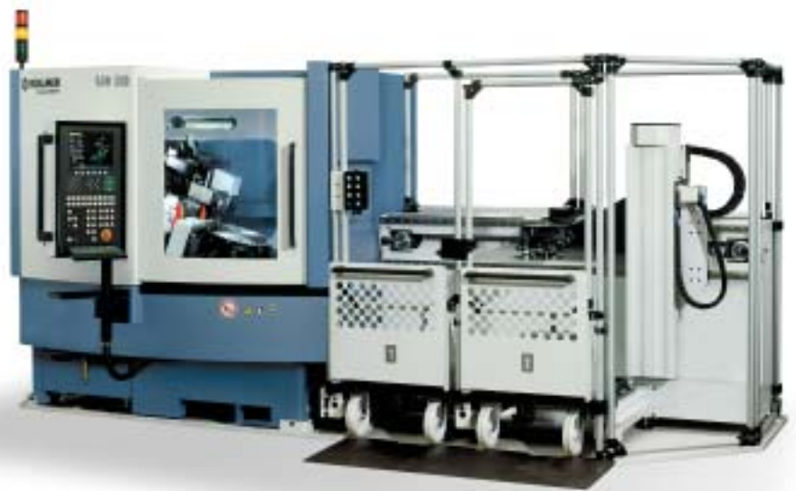
The akemat Service Center with two loading carriages for the fully-automatic machining of approx. 50 saw blades
