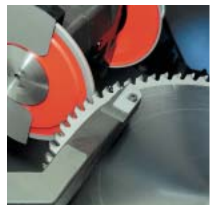
Top grinding with 200mm diameter grinding wheel
