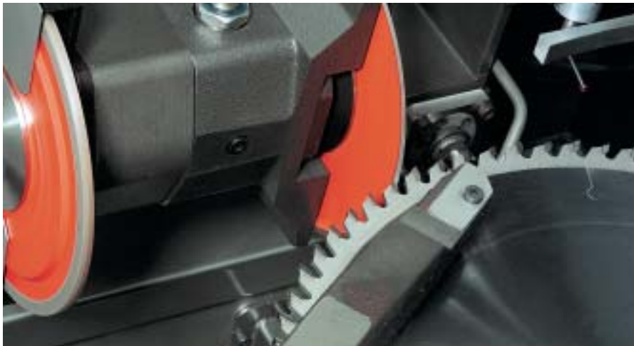
Machining using the akemat grinding principle with inclined saw blade
