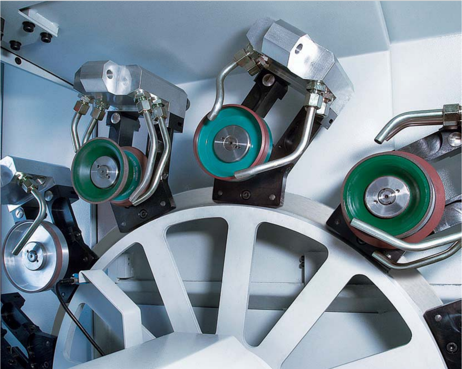
Grinding wheel changer with the Helitronic Vision
