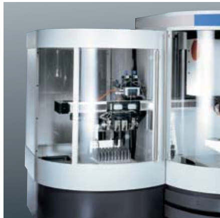
Helitronic Vision with machine-integrated lift loader.
