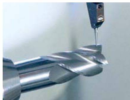
IMS – Rake angle measurement.
