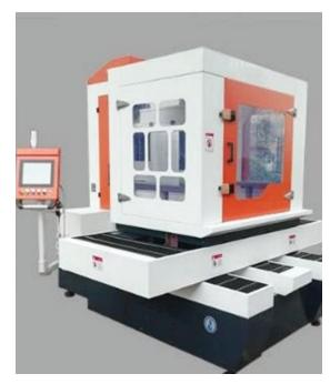
For cutting EDM materials such as graphite, the EDMMax fills the void between a band saw and a Wire EDM. It can perform bulk cutting at speeds that rival a band saw, but achieve accuracy levels such that there is extremely little waste. While it cannot achieve the micron-level accuracy of a Wire EDM, in many cases, the accuracy is acceptable based on the application. The EDMMax can free up the Wire EDM to perform tasks requiring more accuracy.
