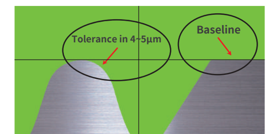
Conventional BallscREW models (Radius tolerance in 4~5μm) Magnification: 120x
