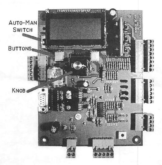
1.1. This new board mounts to the stand-offs already in the control panel, left behind by removal of the old board. The existing wiring plug connectors are 100% compatible. All you need to do to get started is install the board and make the connections. The stroke and speed configuration procedure is new, and will be explained here.
