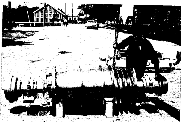
Fig. 23 Jack screws are used to start joint of bowl and bowl head. Conveyor screw is then withdrawn from bowl a short way. Block under bearing housing permits relocation of rigging to maintain balance and finish withdrawing the conveyor.
