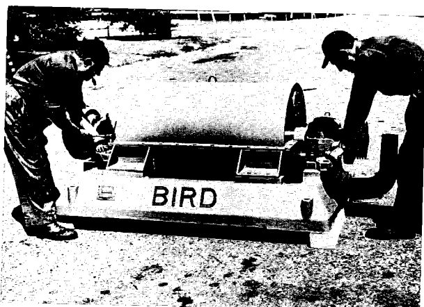
Fig. 20 The feed pipe and the belts have been removed. The gear unit may be left on for quick reassembly if desired. Picture shows removal of bolts so that case top may be lifted off.
