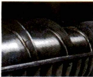
Replaceable wear plates on tapered stainless steel screw shaft
