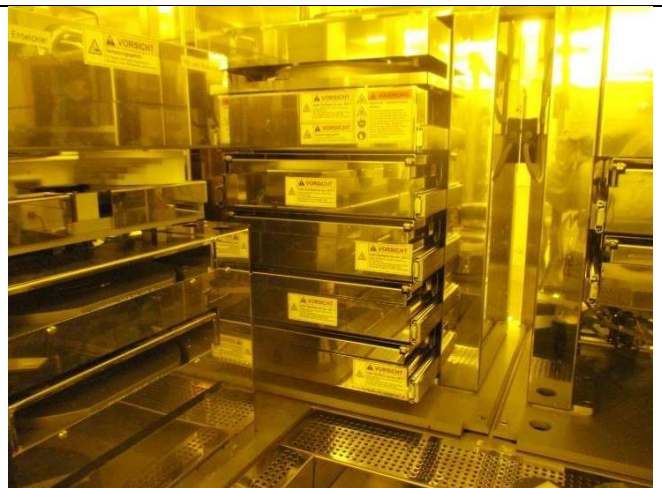
HMDS module (up) + 4 Hotplates (down)
