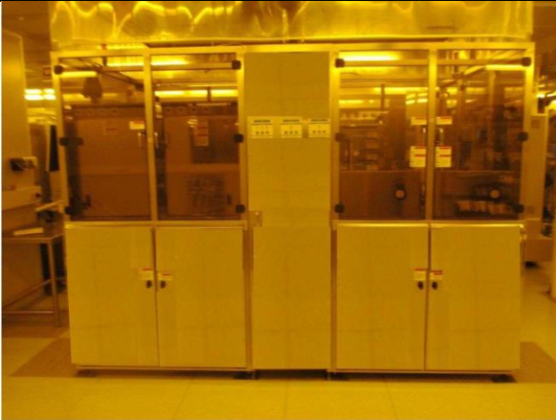
Overall system: left side coating module, right side developing module
