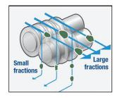
to drop through openings of controlled size. Unlike static screens, however, Jeffrey Rader disc screens continuously move the material across a series of rotating multi-toothed discs. Small particles are shaken loose, larger material is moved on.
