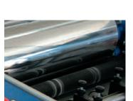
A pneumatically controlled infeed roller presents lightweight and digital output to the laminating and nip rollers where a missing sheet detector helps to prevent unwanted wraparounds.
