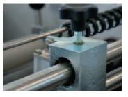
The positioning of the pneumatically controlled perforator overcomes any potential issues caused by poor film roll profiles and allows higher speeds to be maintained.
