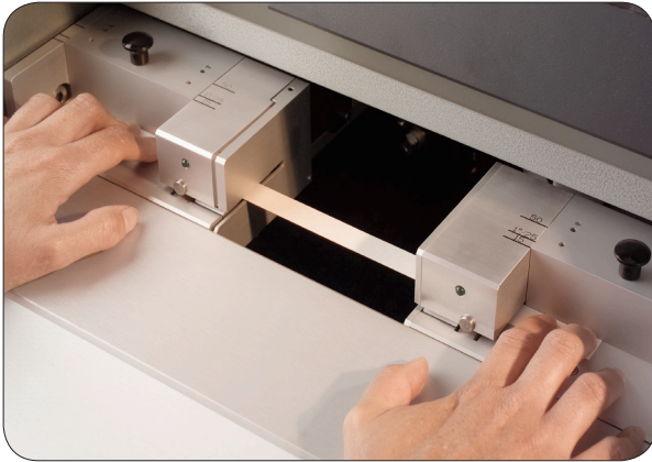
Loading the test piece. A light sensor detects the test piece and measurement starts.
