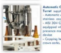
**Automatic Capping** Turret supplied with Automatic AISI 304 stainless cap sorter, - AISI 304 Chute equipped with cap presence monitoring device - Capping head for
