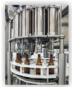
Counterpressure Filling Turret, supplied with 5 Electropneumatic Isobaric valves suitable for filling beer and carbonated drinks into glass bottles.
