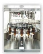
Rinsing Turret supplied with 5 nozzles and equipped with a device for detection of the bottle on the conveyor.
