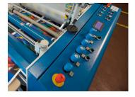
The centralised PLC control panel offers ease of operation and is enhanced with a modem link for remote diagnostics.
