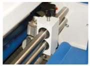
The positioning of the pneumatically controlled perforator overcomes any potential issues caused by poor film roll profiles and allows higher speeds to be maintained.
