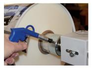
The film mandrel swings out and has an air shaft to speed roll
