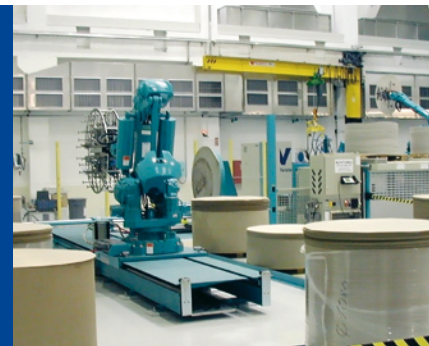
Industrial robot with double grab head to position the outer headers
