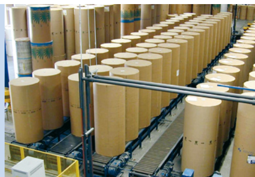
Finished roll warehouse with storage conveyor belts
