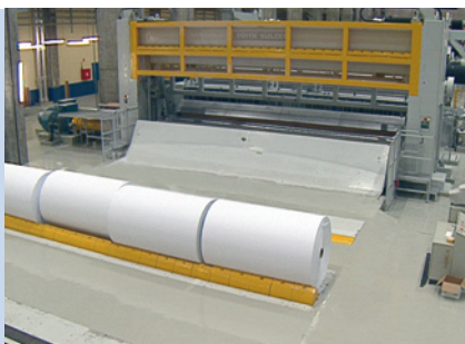
Separation of roll set downstream of the winder
