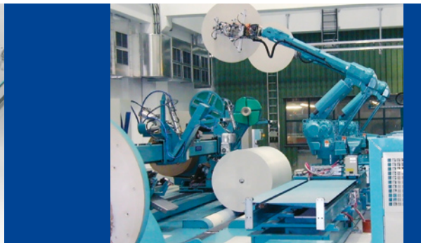
Two robots for simultaneous positioning of both inner headers
