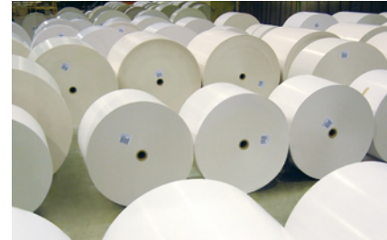
Stopover downstream of the winder – rolls ready for roll wrapping
