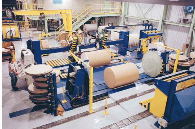
This Twister™ Center wraps up to 60 rolls/hour in a small space
