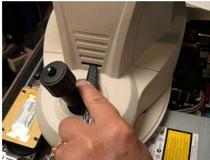
Figure 3.3 Tower Cover Removal
