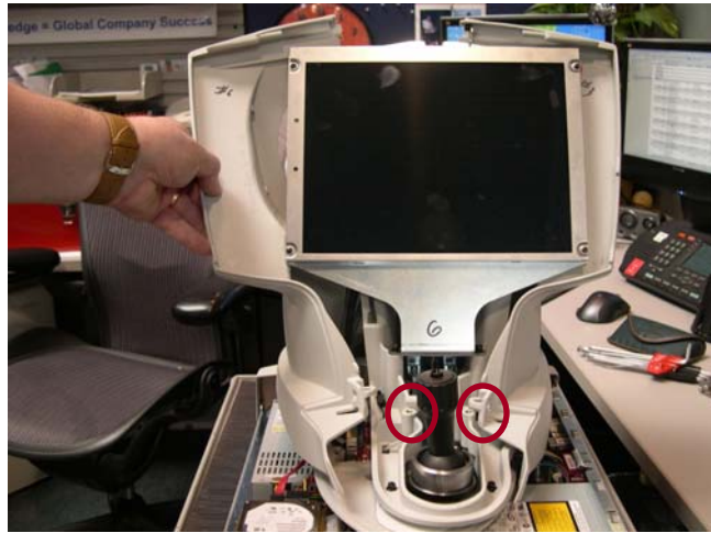
Figure 3.4 Tower Cover Removal
