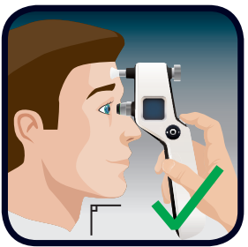
Correct alignment of the tonometer and green probe base light indication.
