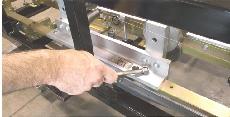
**Figure 50: Removing Tooling Rails**
