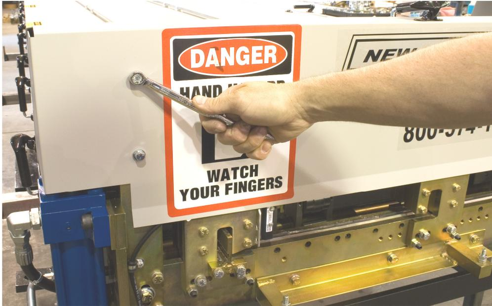
*Figure 64: Removing Shear Cover*
