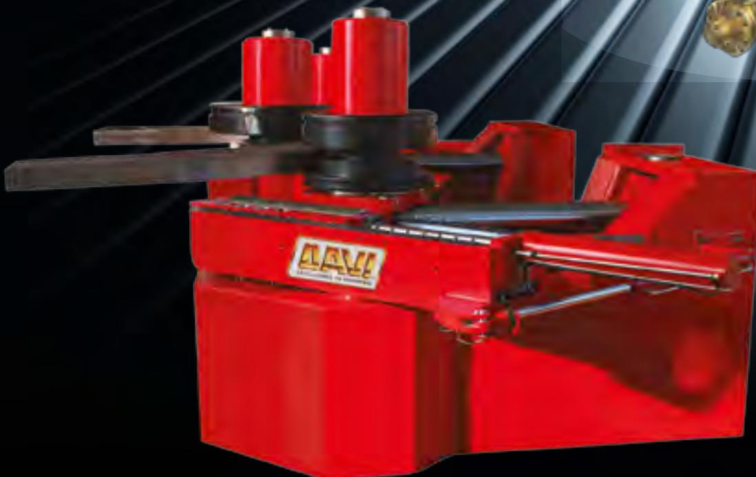
All Machines Equipped With 3-D Guiding Roll
