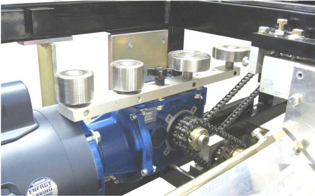
**Figure 71: Unused Inside Box Roller Stored**
