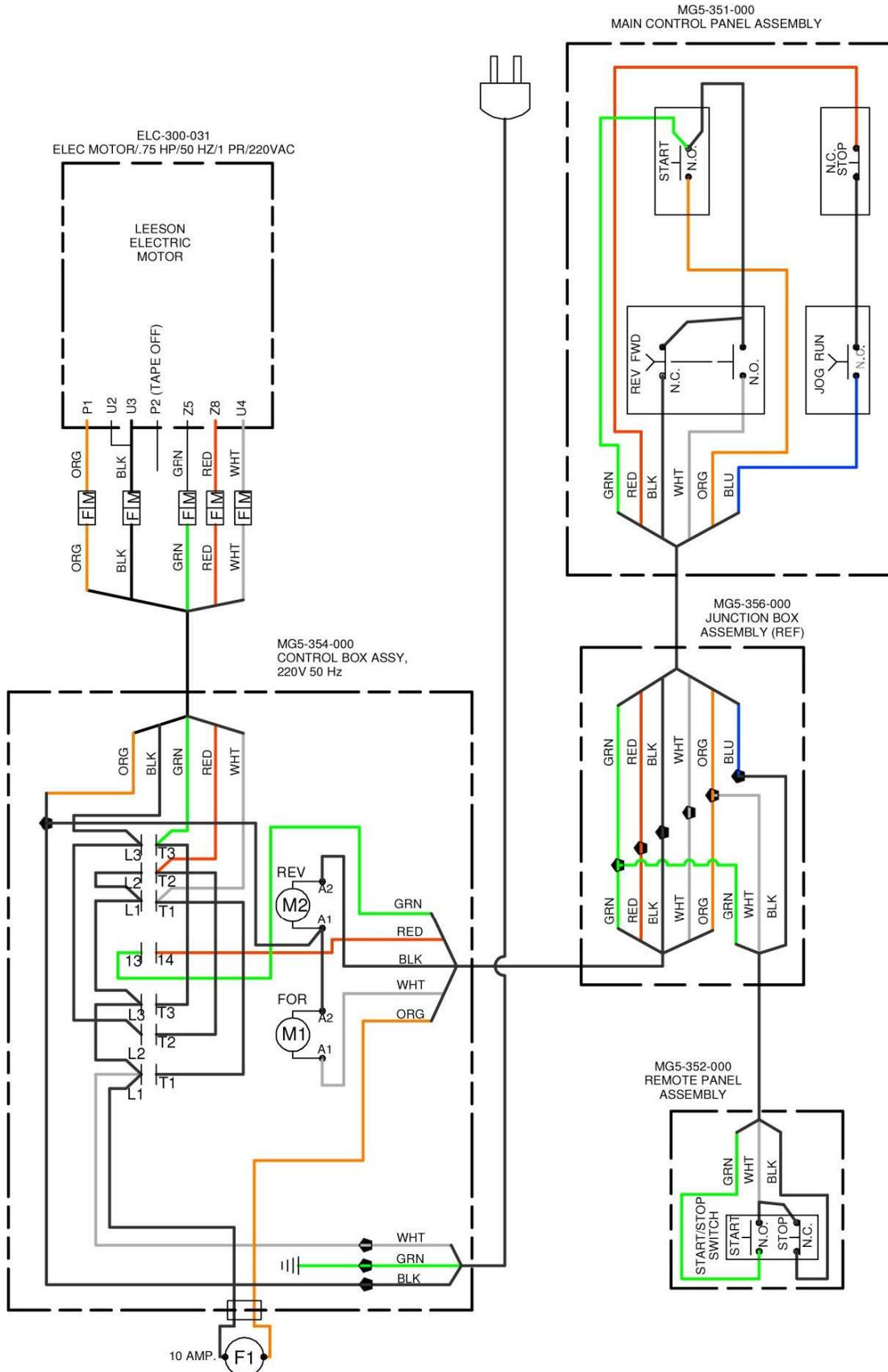
**Figure 90: MG220-50 – 220VAC, 50Hz Wiring Diagram**
