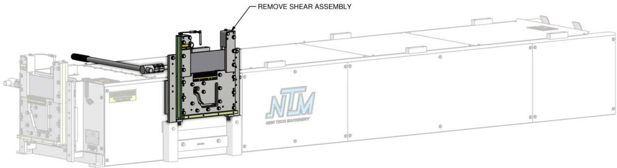
**Figure 41: Remove 6" Shear**
