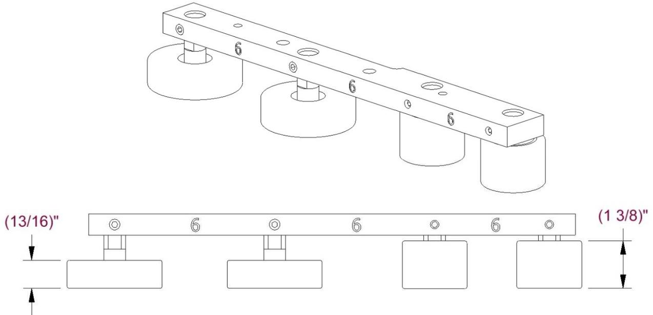
**Figure 54: 6" Roller Bar**
