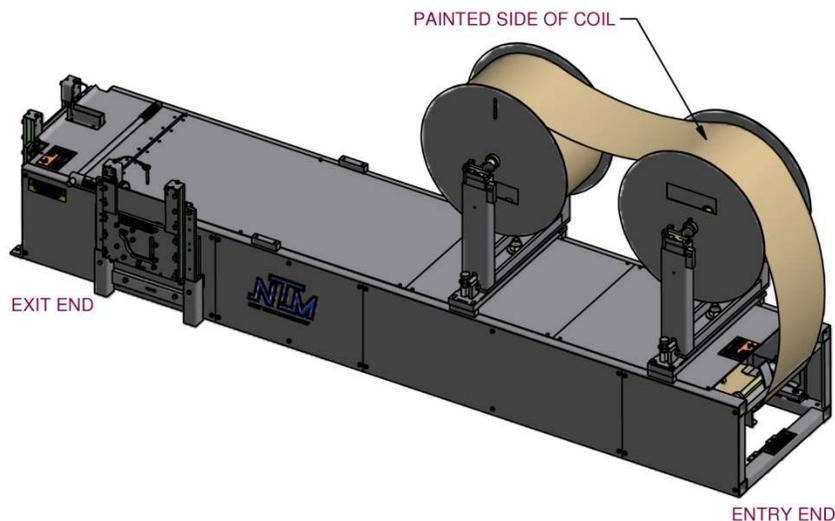
**Figure 13: Coil Routing**
