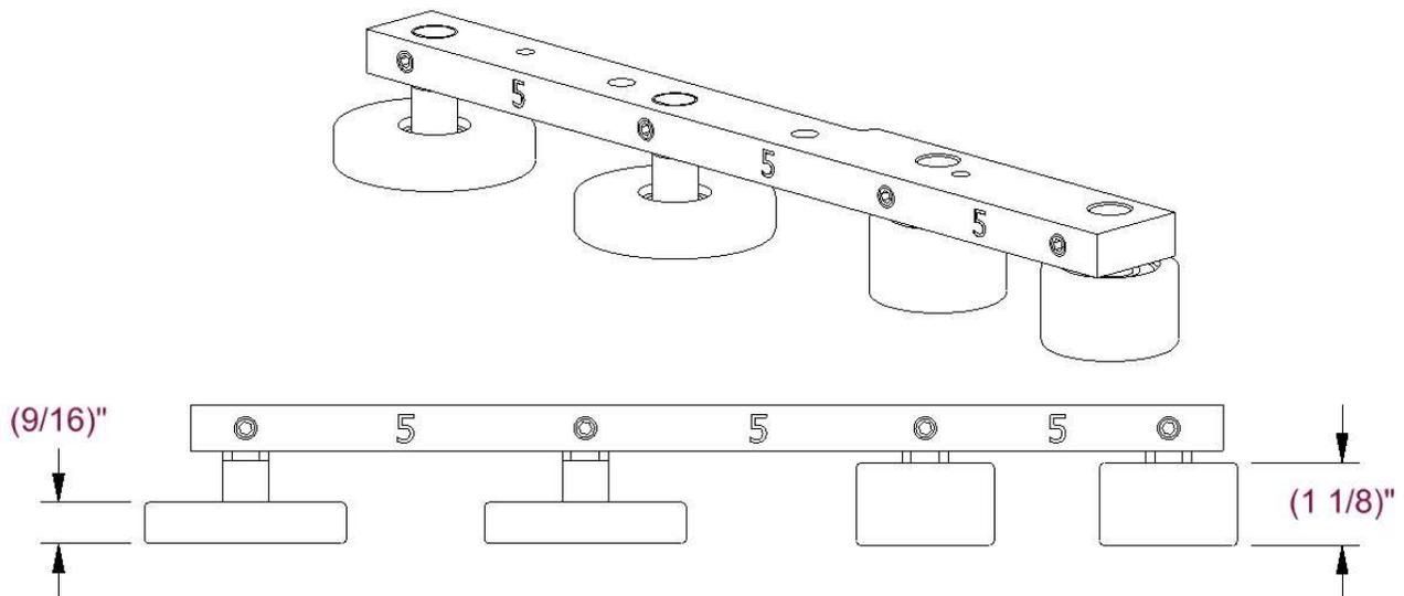
**Figure 70: 5" Roller Bar**
