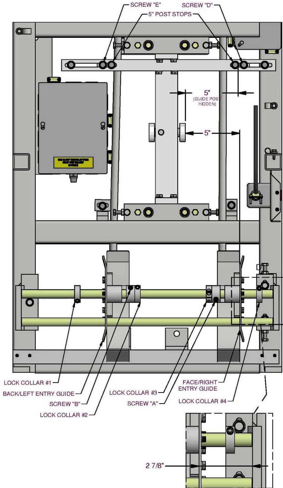
**Figure 17: M56 Entry Guide Setup for 5"**
