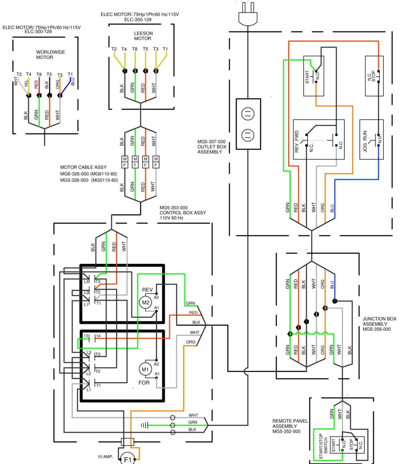
**Figure 88: MG5110-60/MG6110-60 – 110VAC 60Hz Wiring Diagram**
