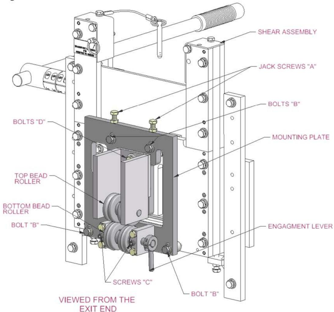
**Figure 82: Bottom Bead Roller Assembly**
