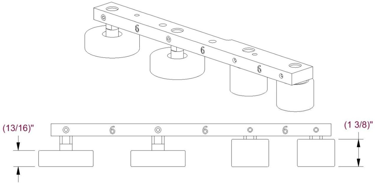
**Figure 67: 6" Roller Bar**
