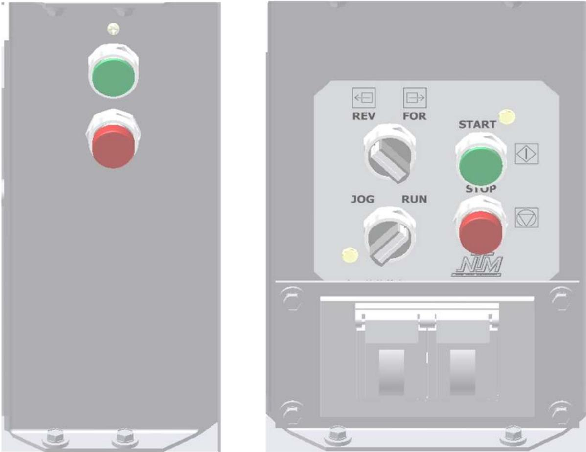
**Figure 5: Remote and Main Control Panels**
