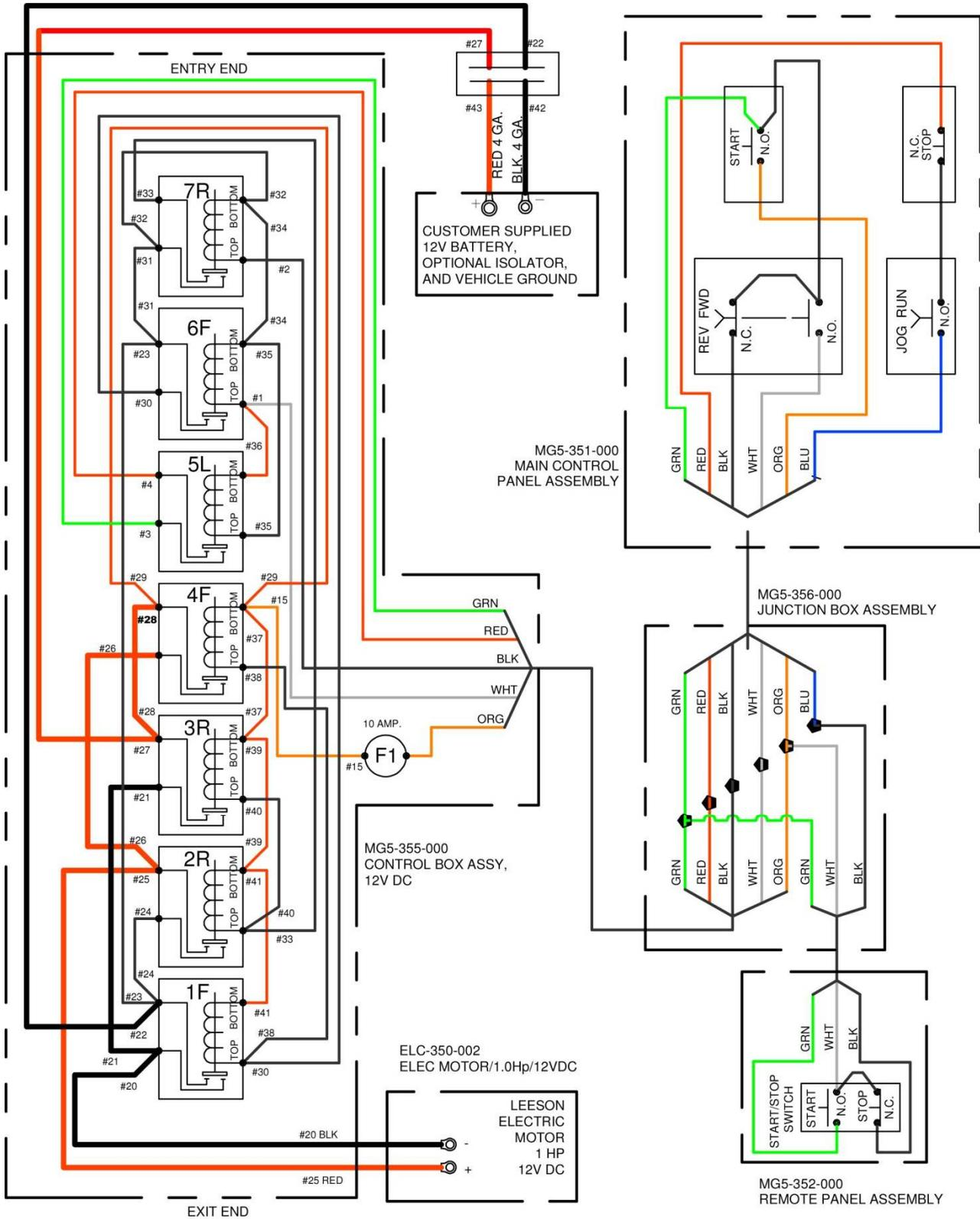
Figure 92: MG12V - 12VDC Wiring Diagram
