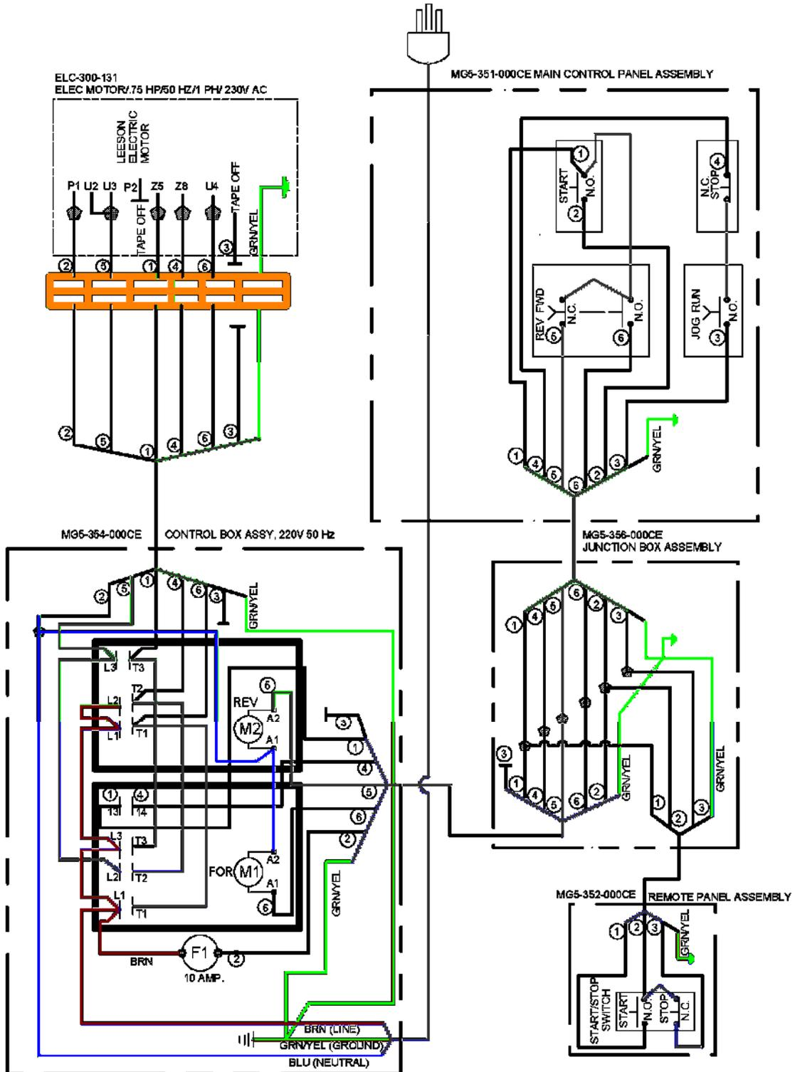
Figure 91: MG230-50CE – 230VAC, 50Hz CE Wiring Diagram
