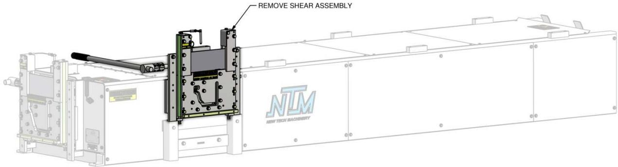
**Figure 57: Remove 5" Shear**
