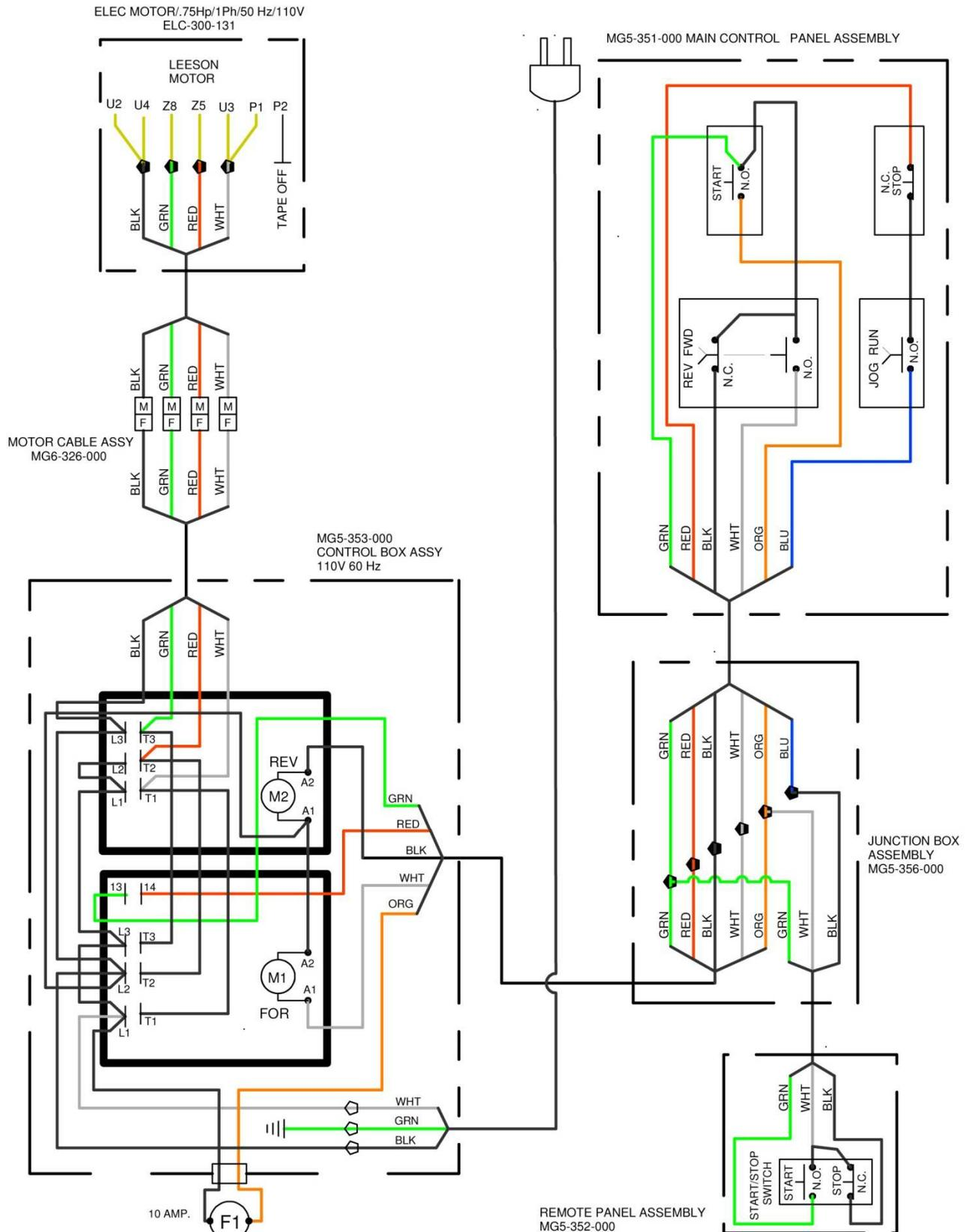
**Figure 89: MG110-50 – 110VAC, 50Hz Wiring Diagram**
