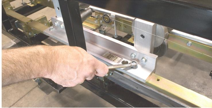
**Figure 41: Removing Tooling Rails**
