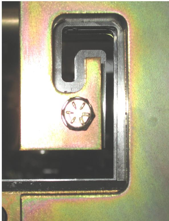
**Figure 39: Exit Die Adjustment**
