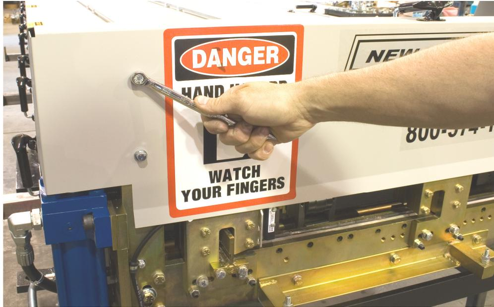
*Figure 59: Removing Shear Cover*
