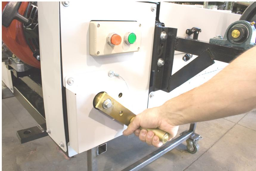
**Figure 54: Tooling Rail Adjustment Handle**
