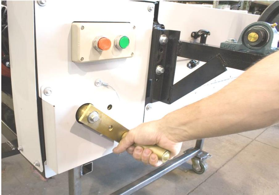
**Figure 24: Tooling Rail Adjustment Handle**
