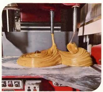
Installation of a TZ.40 between an IM.30 batch kneader and an AL.60 batch feeder in the Candy Servomatic line will give you automation of the sugar pulling operation and hence a saving of labour costs.
