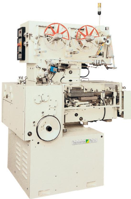
**Forming, cutting and wrapping machine for chewing gum or bubble-gum-products in double point end fold with comic strip as inner wrapper**
