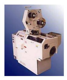
The **750W** is a cut and wrap machine specially designed for 'Whirl', 'Kiss' or 'Face-cut' pieces, with a design showing in the centre of the product. The machine can be produced for either double twist or fold wrapping styles, although it is most common to have double twist style, to show off the product to its best effect.
