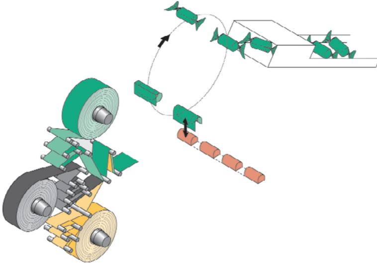
Wrapping machine for deposited or enrobed chocolate products with or without center-filling in double twist wrap (or »protected twist« upon request). The products are aligned by means of a feeding and separating station and are conveyed to the wrapping station by a feeding belt. A low accumulation pressure of the product in the feeding section is achieved by an automatic speed control.
