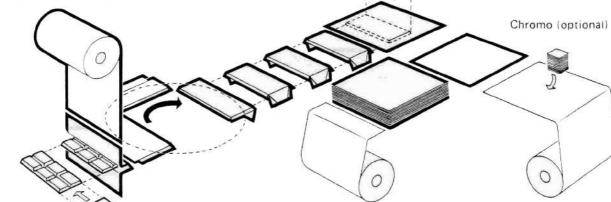
Outer wrap from stack, or from reel, photo-electrically registered.
