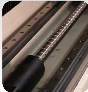
High performance dual ball screw drives with optional glass scales.
