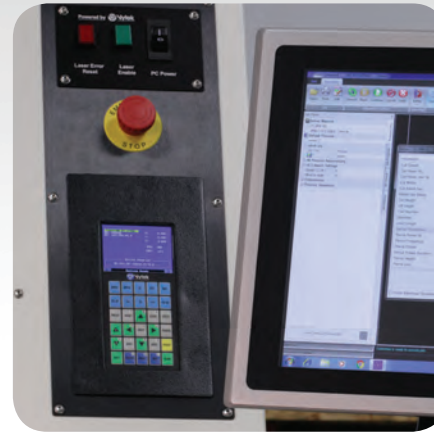
Integrated control technology running with an advanced, touch-screen user interface.
