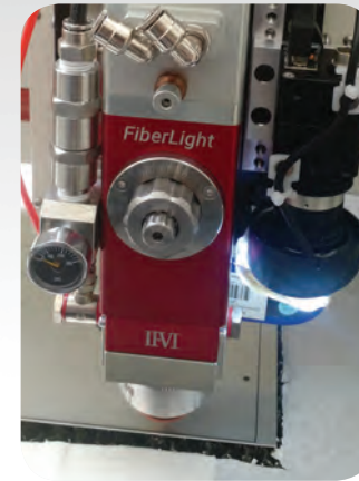
Vision alignment option for precise part orientation.
