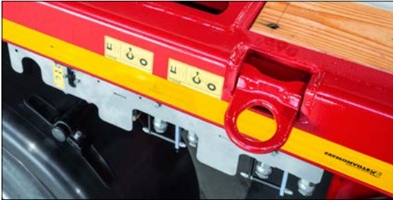
Outwardly hinged lashing rings
