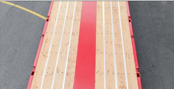
Timber floor framed in aluminium omega profiles
