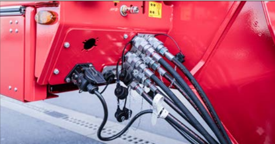
Hydraulic screw couplings
