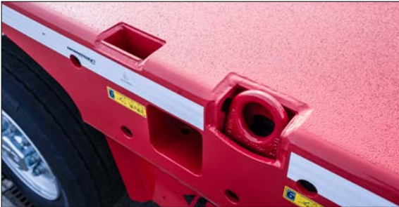
Lashing rings and stake pockets
