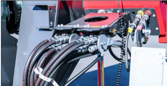
Multiple hydraulic couplings
