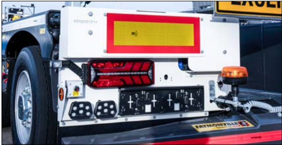
Tail lights for central bogies
