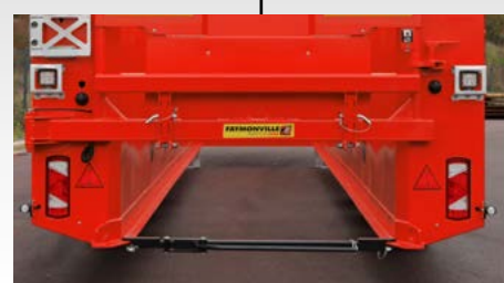
Cross-bar at the rear with eccentric closing
