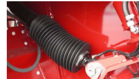
Standard equipment: Protection jackets on the hydraulic cylinders
