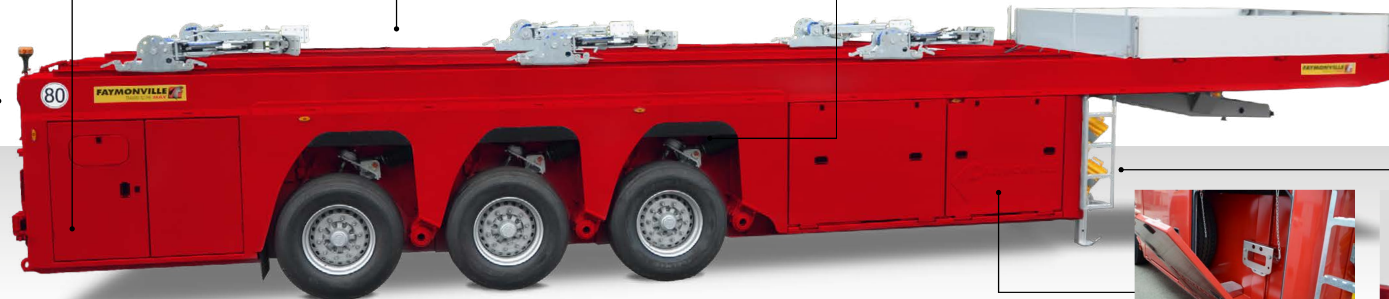
Standard equipment: In front of the axles, on both sides, removable lateral protections *
