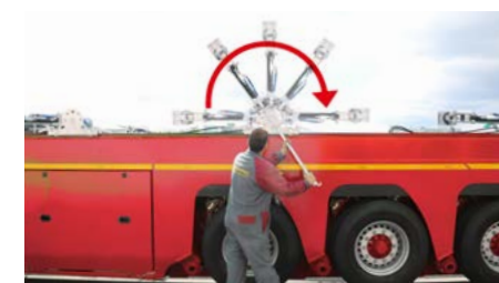
Handling of the load securing systems easily carried out from the ground
