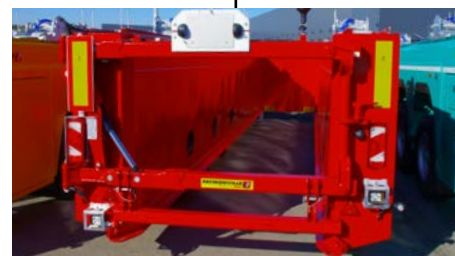
Vertically adjustable rear door, hydraulically activated
