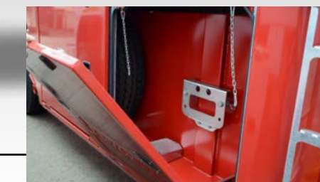
Standard equipment: In front of the axles, on both sides, removable lateral protections *
