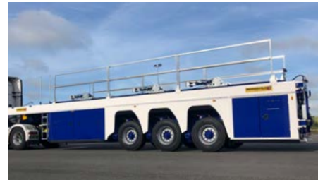
Removable hand rail on the lateral beams
