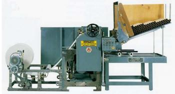
Heavy plain, printed, waxed, or coated papers, building papers, asphalt papers, and protective papers, plastics, vinyls, HDPE, and aluminum foils – supported and unsupported – are all quickly handled by the Schultz Type XZ. This rewinder automatically feeds the web, starts winding around the core without tape or adhesives, cuts off accurately to the desired length, and deposits finished rolls on the conveyor. Exact roll tension assures high product quality.
