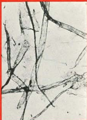
Photomicrograph of fully repulped furnish shows excellent separation of fibers without damage or cutting.
