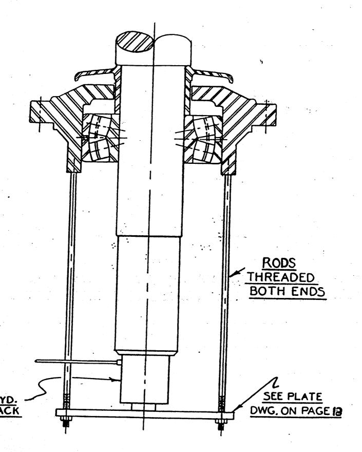
RECOMMENDED REMOVAL OF BOTTOM BEARING & HOUSING
