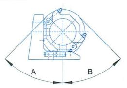
The marking arrow is located on the front side of the force sensor. The direction of the resulting force of the felt/wire tension should correspond to the direction of the arrow.
