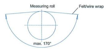
■ The resulting force of the felt/wire wrap can deviate a maximum of ±50° from the measuring direction of the force sensor.
