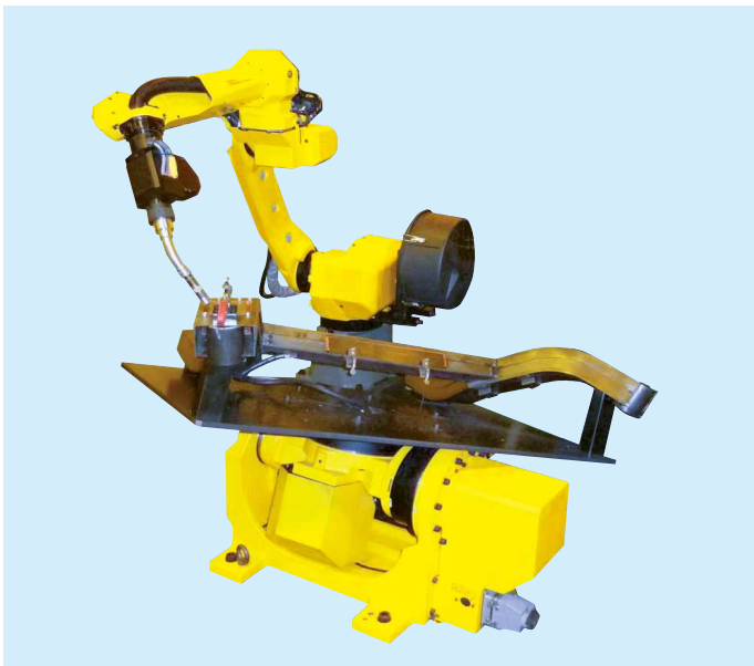
Automobile part arc welding with Servo Torch
