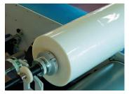
Both top and bottom mandrels are of swing out design for easy film loading and allow lateral film adjustment to be made on the run.
