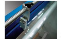
The Comet is equipped with adjustable side slitters to trim the web.
