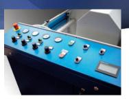
The easy to use plc controls incorporate a modem link for remote diagnostics.
