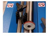
The positioning of the perforator overcomes any potential issues caused by poor film roll profiles and allows greater speed and decurl angles minimising web breakage.
