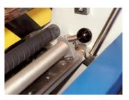
A decurl bar, which may be altered on the run, is fitted to assist in giving a flat result when laminating on one side only.
