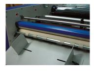
The adjustable burster automatically separates sheets. A cushion of air supports the sheet as it is delivered into the catch tray.
