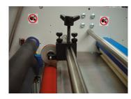
The positioning of the perforator overcomes any potential issues caused by poor film roll profiles and allows higher speeds to be maintained.
