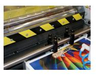
An infeed roller presents lightweight and digital output to the laminating and nip rollers where a no sheet detector helps to prevent unwanted wraparounds.
