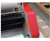
Colour coded mandrels ensure that core grips always face the correct way to tension the film for a flat result.
