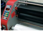
Heated shoes provide a rapid warm-up and consistent heat source for both high and low melt films.
