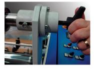
The madrel has a hinged support and film can be adjusted laterally on the run to minimise waste and down time.
