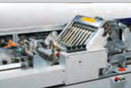
Feeding system 434 with four automatic fold plates
