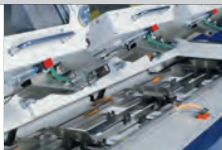
Easily accessible document track because of swing-mounted insert feeders
