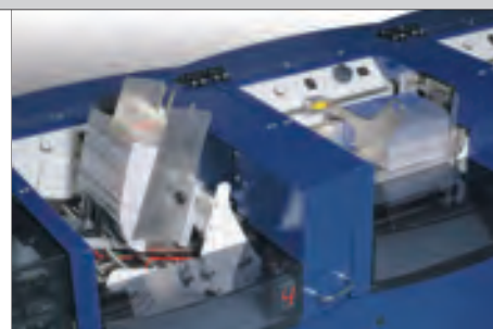
Insert station with friction and suction feeder
