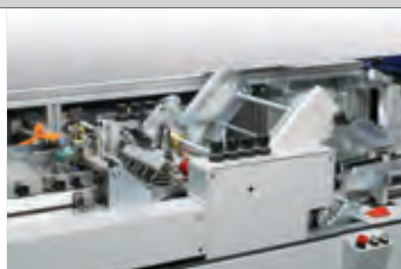
Feeding system 434/428 with transfer module without fold plates for short forms applications
