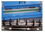
The flying knife separator separates OPP, Nylon and Polyester films with ease whilst a cushion of air supports the sheet as it is delivered into the catch tray.
