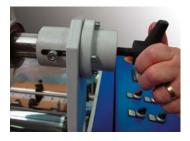
The mandrel has a hinged support and film can be adjusted laterally on the run to minimise waste and down time.
