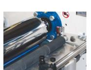
An infeed roller presents lightweight and digital output to the laminating and nip rollers where a missing sheet detector helps to prevent unwanted wraparounds.
